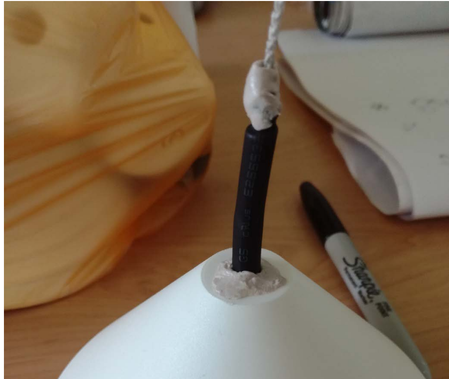
Figure 10: Step 9 – Use some modelling clay to seal the hole where the tube enters the funnel and the upper part of the heat shrink tube if necessary.
