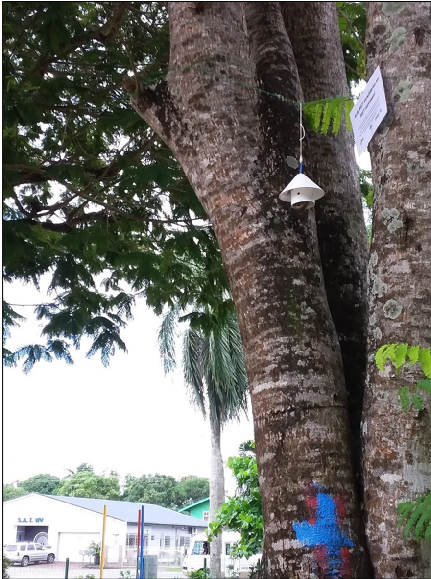
Figure 20: Air temperature recording drops utilised within this study and the wider TBIS twinning project.
